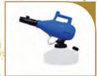
(CVR-001) Fogging machine Tank Capacity: 4.5L ,Power:220V/50Hz 1100W , Atomization Volume: 150- 260ml/min(adjustable) Particle Size: 10-150µm (adjustable) Effective range: 6-12m
